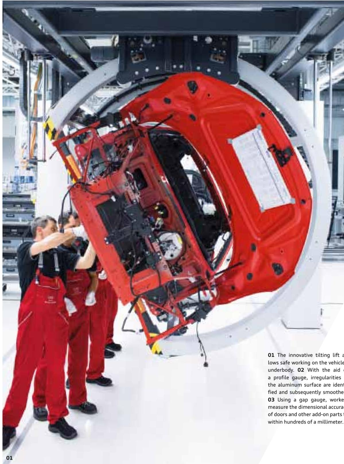
**01** The innovative tilting lift allows safe working on the vehicle's underbody. **02** With the aid of a profile gauge, irregularities in the aluminum surface are identified and subsequently smoothed. **03** Using a gap gauge, workers measure the dimensional accuracy of doors and other add-on parts to within hundreds of a millimeter.
