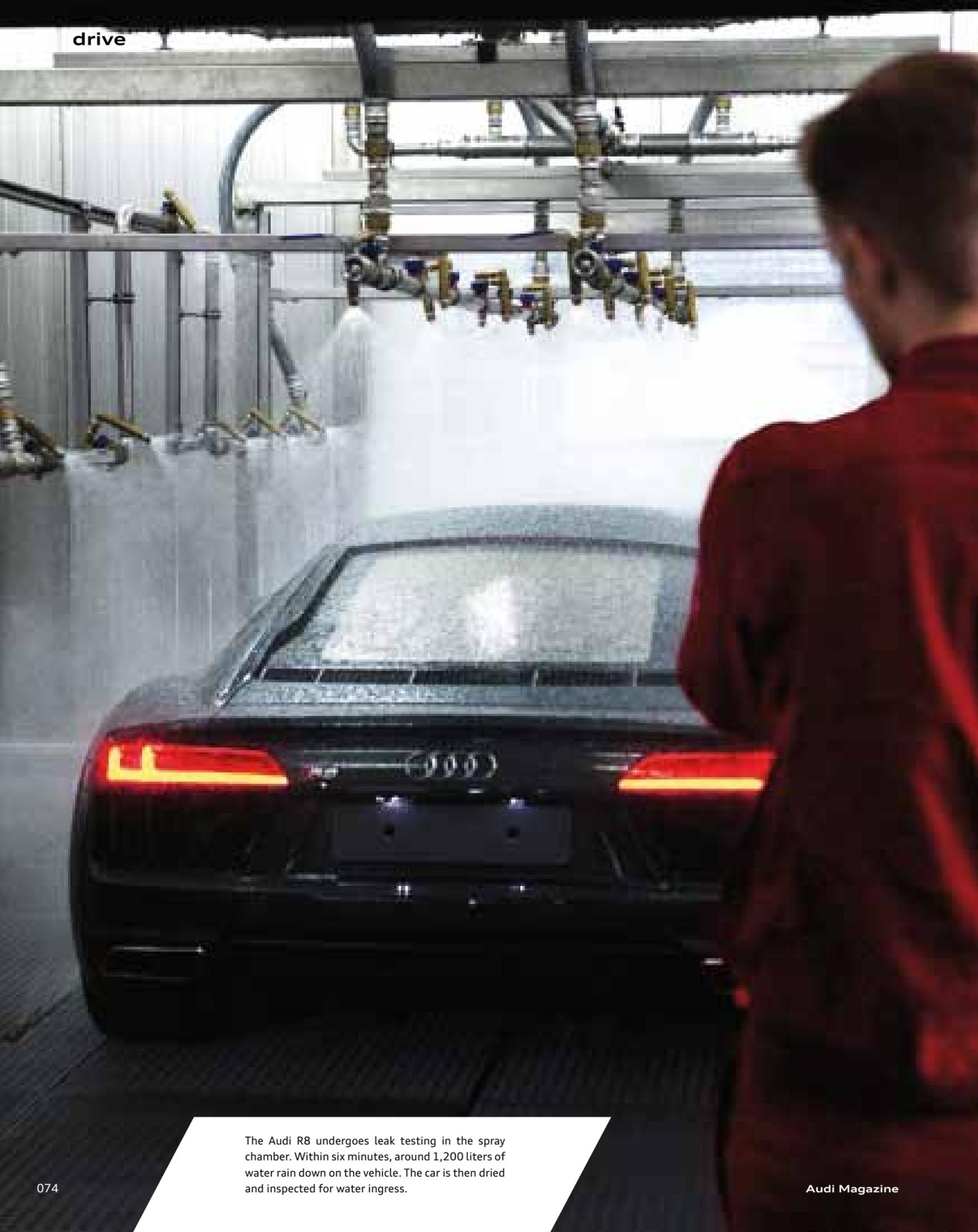
The Audi R8 undergoes leak testing in the spray chamber. Within six minutes, around 1,200 liters of water rain down on the vehicle. The car is then dried and inspected for water ingress.
