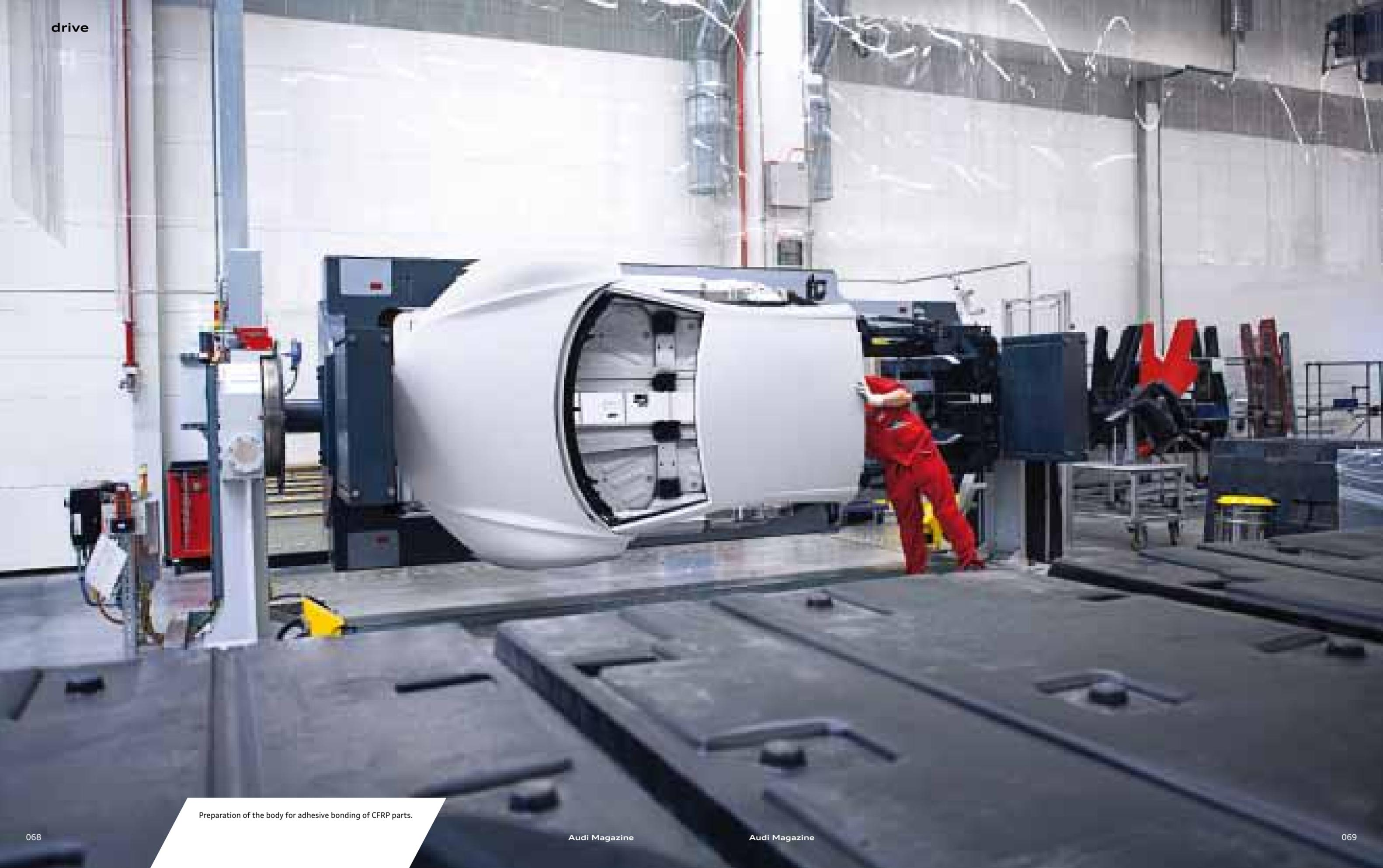
Preparation of the body for adhesive bonding of CFRP parts.
