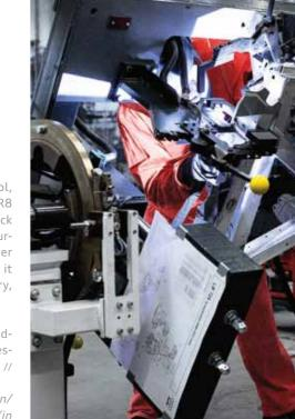
Just as Bianca Kreis is responsible for visual quality control, test driver Sadik Morina ensures that everything inside the Audi R8 works as it should. He drives the vehicle over a vibration test track in order to pinpoint unusual noises or other irregularities. "During the subsequent road drive, we test the Audi R8—also at higher speeds—to make sure everything's OK," explains Morina. "Then it goes through a final inspection. When it finally leaves the factory, it's really something special."
