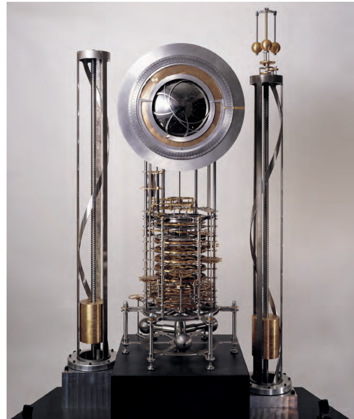
The concept of the clock is based on an electromechanical construction. A torsional pendulum sets the clock pulse. Brian Eno developed the algorithm that is the basis for the melody of the chimes. The finished artwork is to be installed deep underground in a Texan tunnel, protected against vibrations and external influences.
